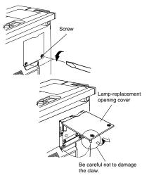
2 Loosen the screws, raise the handle, and pull out the light-source lamp.
